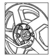
Use the wheel wrench to remove the wheel nuts securing the spare tire.
